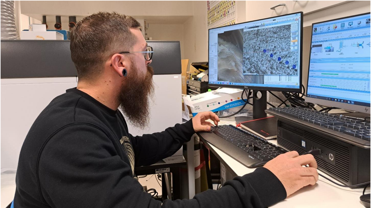
Fig. 1. Programming of a transect for the laser ablation analysis with the Neptune Plus software.
