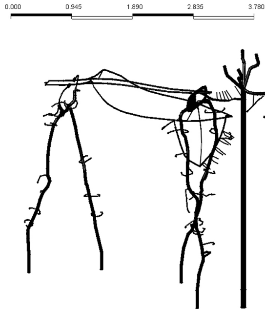
Fig. S5 - The Finite Element model of the metal structure supporting the mammoth.
