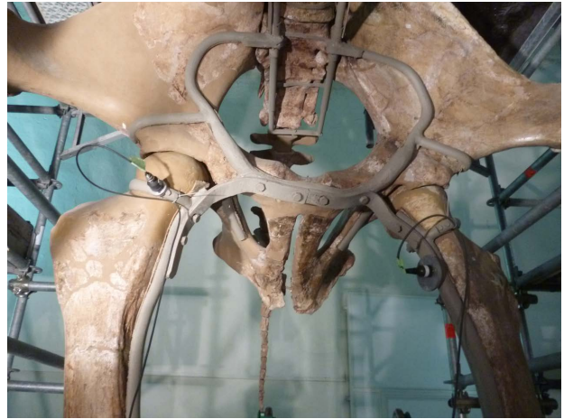
Fig. S6 - View of some of the acceleration sensors.
