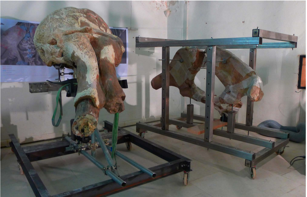
Fig. S9 - Support systems with specific structures were used for the skull and pelvis.
